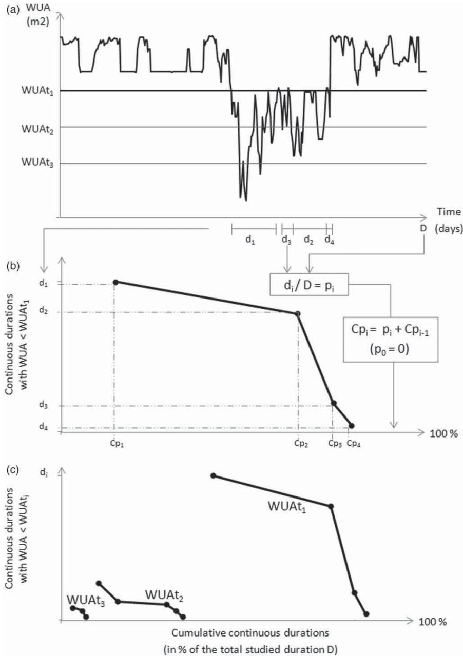
Figure 3. Construction of continuous under-threshold curves from the habitat time series curves.
