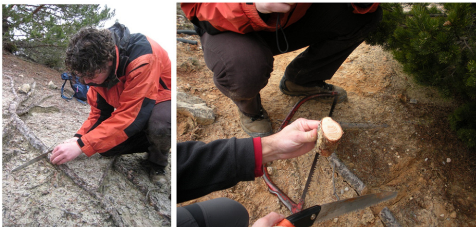
Fig. 4. Sampling exposed root by sheet erosion oriented according to the slope direction with a hand saw.
