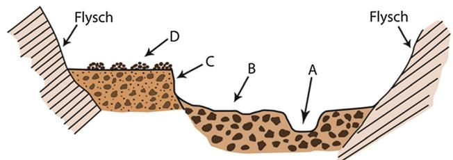
Figure 4. Idealized organization of the sedimentary environments in the upper torrential reach of the Ijuez River. A: active channel; B: active alluvial plain; C: fluvial terrace; D: debris flow deposits. The width of the valley bottom is approximately 150 m. The difference in height between the fluvial channel and the upper part of the terrace is 4 m. This figure is available in colour online at [wileyonlinelibrary.com/journal/ldr](http://wileyonlinelibrary.com/journal/ldr).
