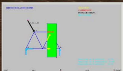
Example 1: Calculation of tension forces in a framework with the sections method
